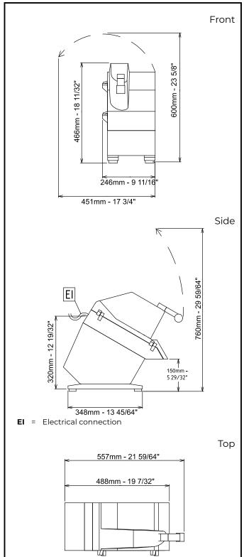
Electric Supply voltage: 602256 (DTR24SNU) 115 V/1N ph/60 Hz Electrical power, max: 0.64 kW **Total Watts:** 0.64 kW Capacity: Performance (up to): 450 kg/hour Performance (up to) 992 lbs/cycle Key Information: External dimensions, Width: 9 11/16" (246 mm) External dimensions, Depth: 21 15/16" (557 mm)
